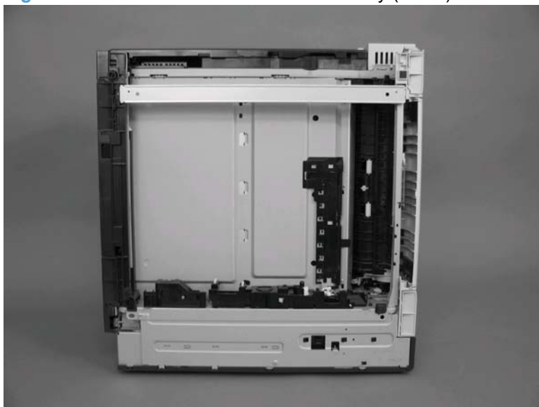
Figure 2-53 Remove the lifter-drive assembly (1 of 3)
