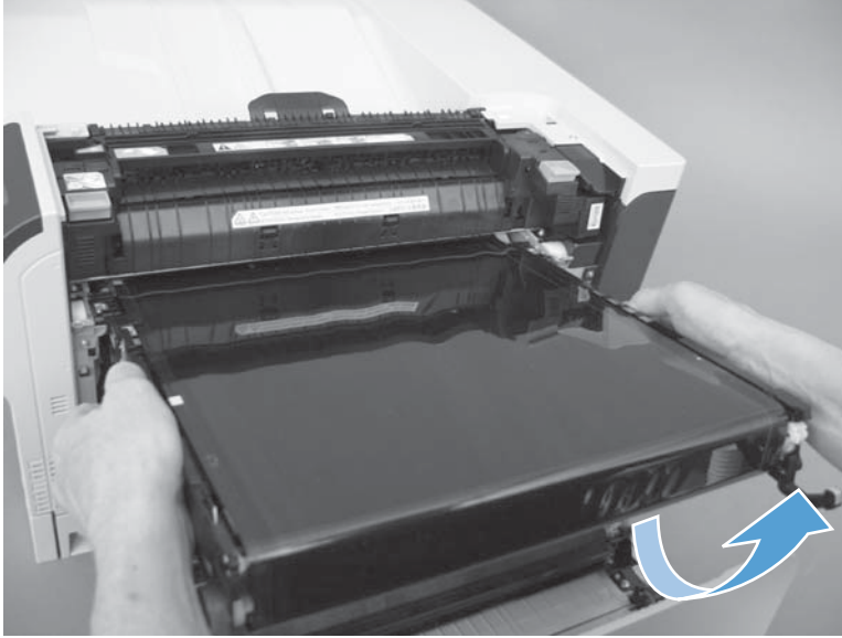
Figure 2-18 Remove the intermediate transfer belt (3 of 3)
