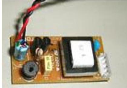
Figure 4.6 Lamp inverter circuit
